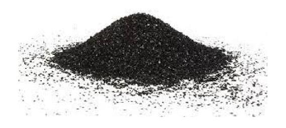
GAC Fines - Small particles of carbon called carbon "fines" are normal to be present in a new GAC filter when it is first installed.
