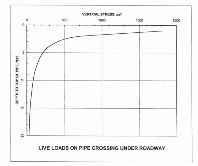
Note: 1. The vertical stress was estimated using AASHTO HS20 truck axle loadings on paved surfaces (Reference: ASCE 15-98, "Standard Practice for Direct Design of Buried Precast Concrete Pipe Using Standandard Installations").
