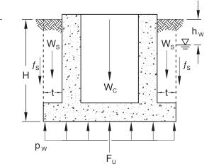
cohesive soils:  $f_{S_j} = \alpha c_j \leq 3,000 \text{ psf}$ cohesionless soils:  $f_{S_j} = 0.75 \text{ K}_S \sigma_{V_j} \tan \delta_j$
