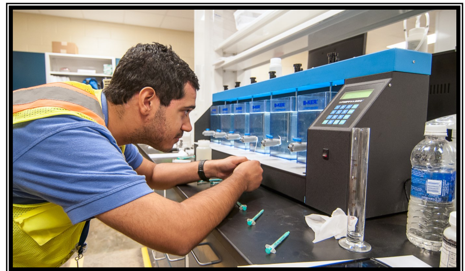
Surface Water Facility operator inspecting sludge floc produced during start-up and commissioning of the Surface Water Treatment Facility
