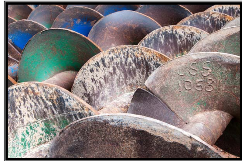
Above: Auger Bits Used For Tunnel Excavation
