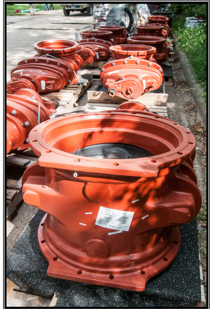
Butterfly valves along Transmission Line Segment W3A
