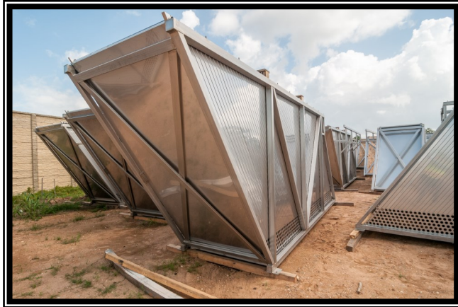
Plate settlers to be installed at the Pretreatment Facility
