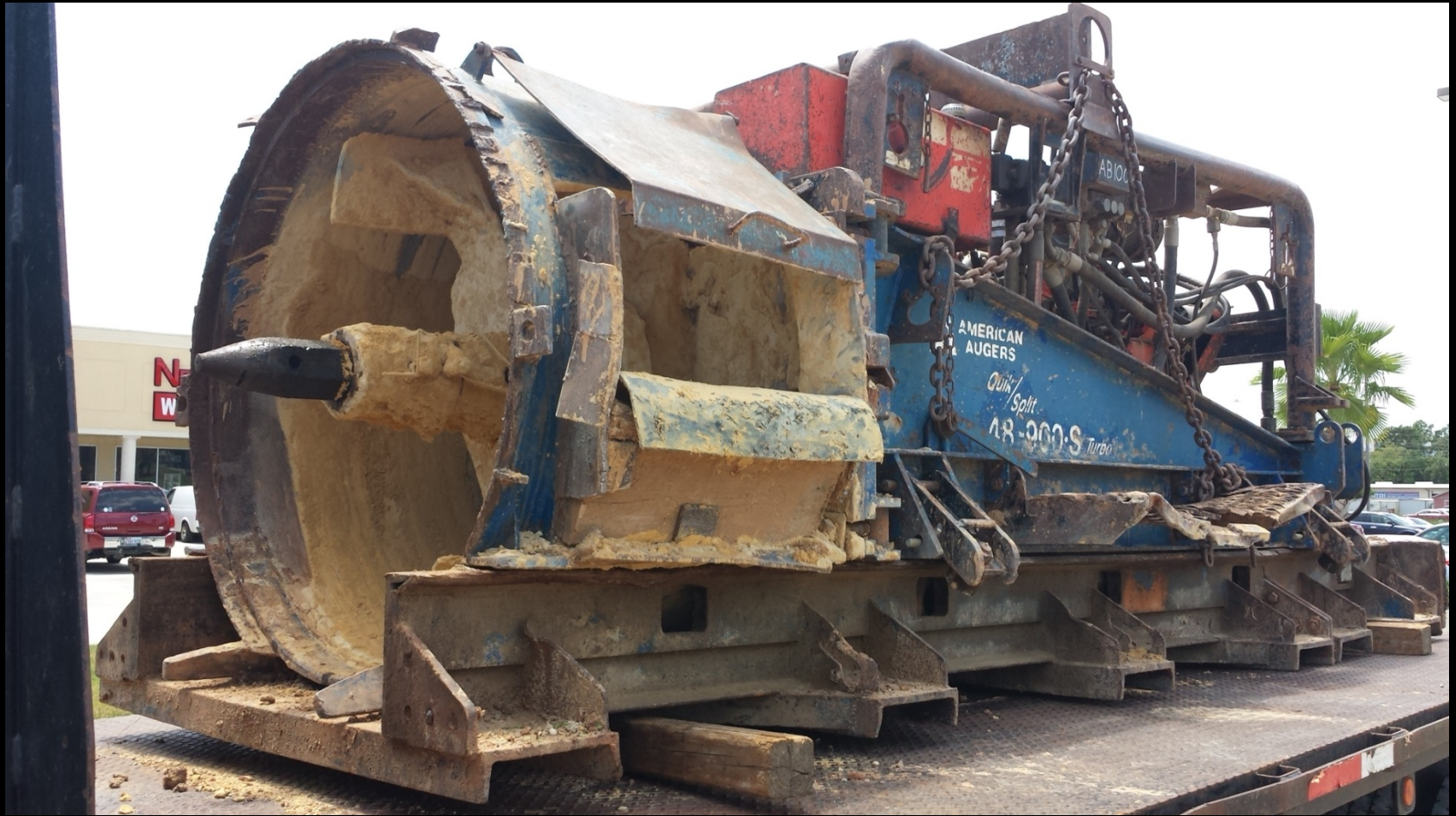
36-inch dry bore auger machine for Rayford Road Crossing
