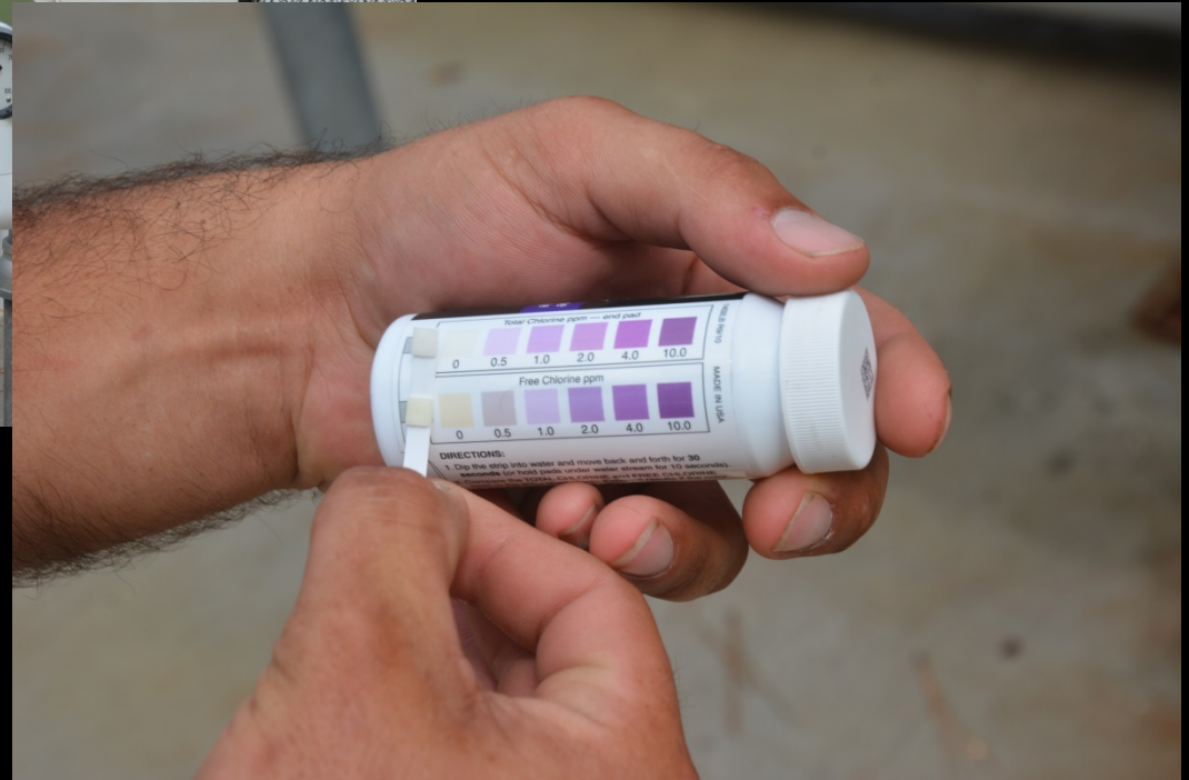
Verification of dechlorination at Water Receiving Facilities
